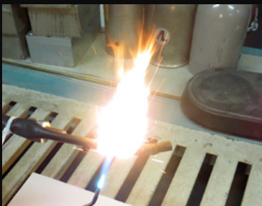
30-second flammability test for certification in accordance with DNV GL
